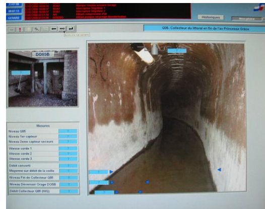
Visualization of the littoral collector of the Princesse Grace Avenue on PcVue
